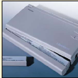
Just like the grown-ups: the Libretto 100CT has slots for two PC Cards Type II or one Type III. A high-capacity battery lasts for up to 5 hours of mains free operation.
