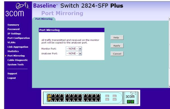
To set up traffic monitoring for a port:
