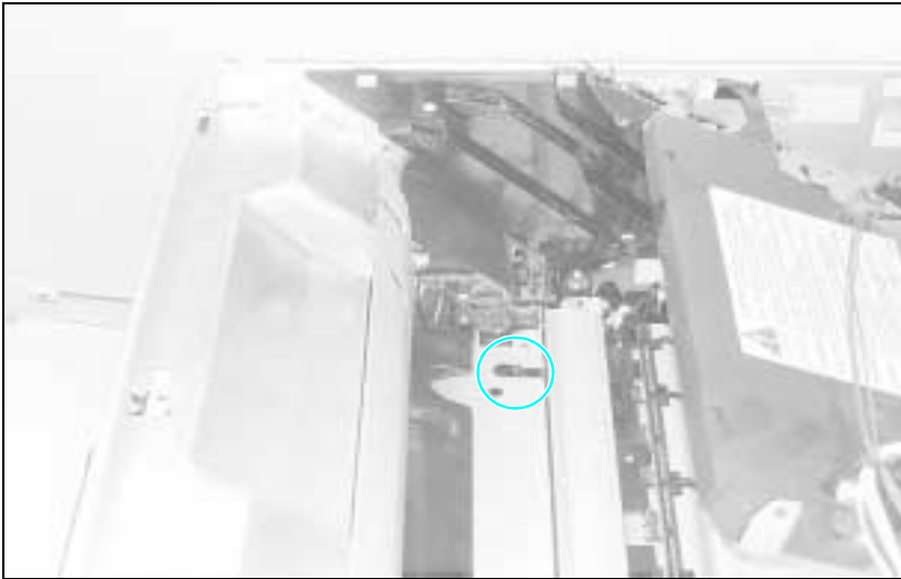
Figure 7-4 PS1 Input/Registration Sensor
