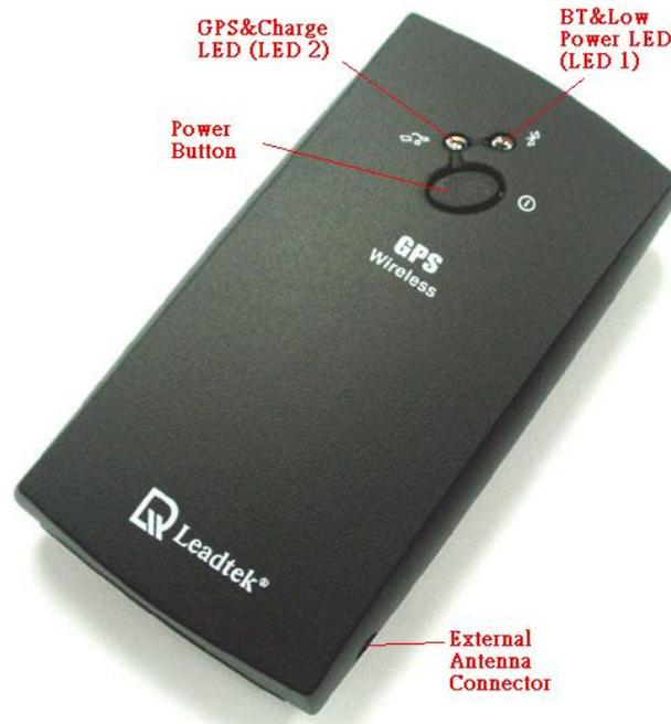
The Bluetooth GPS has two LED light which each has two colors. One is GPS & Charge status LED, that is named LED 2, and the other is Bluetooth & low power status LED, that is named LED 1. The status table of LED shows as follows:
