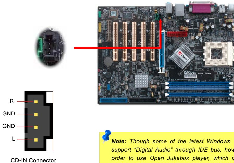
**Note:** Though some of the latest Windows versions support "Digital Audio" through IDE bus, however, in order to use Open Jukebox player, which is driven under BIOS, it is a **MUST** to insert audio cable to CD-IN connector on the motherboard.
