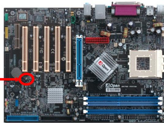
**Warning:** Do not install or remove the DIMM module or others devices when the STBY LED lights on.
