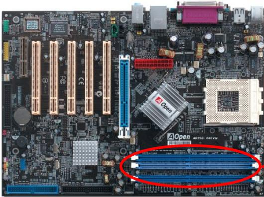
**Warning:** This motherboard supports DDR RAM. Please do not install the SDRAM on the DDR RAM sockets; otherwise, it will cause serious damage on memory sockets or SDRAM module.
