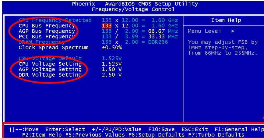
Also, the same keys help you adjust the voltage of CPU and DDR settings. Some values may change while you adjust the settings. You can press “F10” to save the changes you’ve made.
