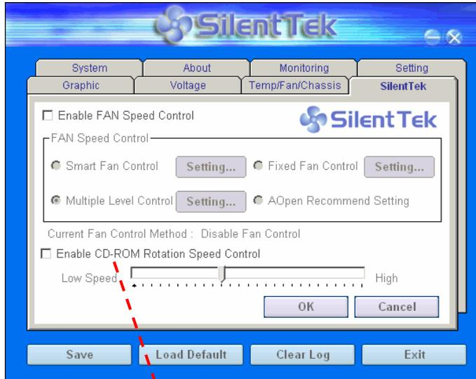
**CD-ROM Rotation Speed Control:** by enabling the CD-ROM Rotation Speed Control, you can adjust the rotation speed of your CD-ROM. When you set the speed to high level, the CD-ROM will work at its fastest speed and it will run at basic required speed while you set the value to low speed.
