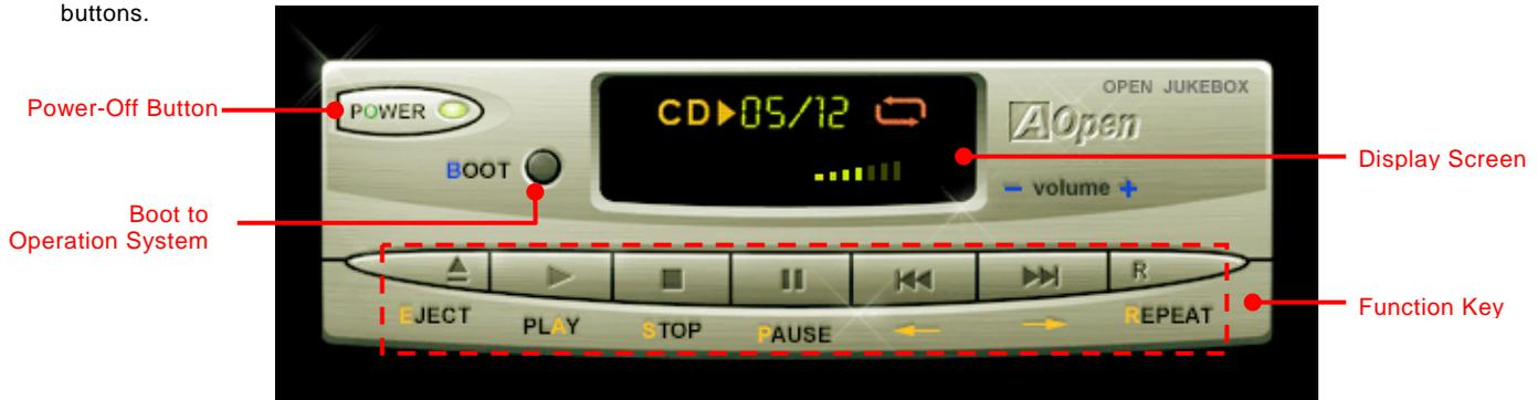
**Power:** Pressing **O**, to directly power off your computer with no hassle of entering Windows Operation System.
