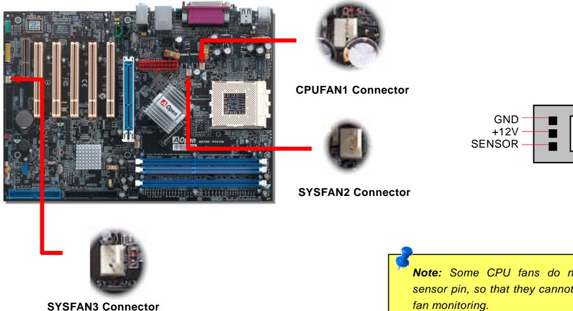
**Note:** Some CPU fans do not have sensor pin, so that they cannot support fan monitoring.
