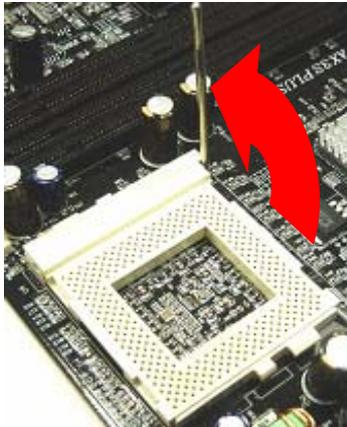
2. Locate Pin 1 in the socket and look for a black dot or cut edge on the CPU upper interface. Match Pin 1 and cut edge, then insert the CPU into the socket.
