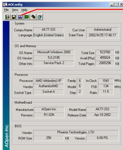
1. The system page shows the detail information of the motherboard, the operating system, the processor, and BIOS version.
