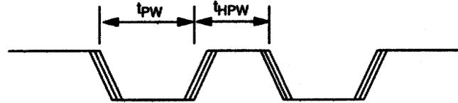
If during any pushbutton activity the STR input is activated, pushbutton operation will be suspended until the storage of EEPROM has been completed. Once complete, pushbutton inputs, if still active, will resume from the point of suspension. Command initiated storage operations will require a minimum of 4 ms to complete the storage operation. This 4 ms is measured from the rise of STR input (see Figure 5).
