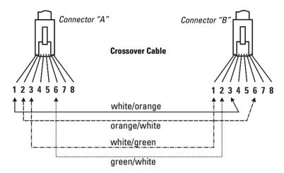
**Note** Pins 1 and 2 on connector "A" *must* be wired as a twisted
