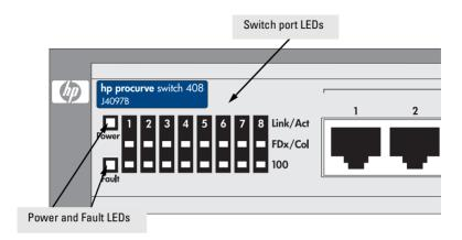
When the switch is powered on, it performs its diagnostic self test. The self test takes approximately 3 seconds to complete.
