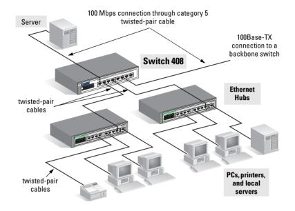
In general, the Switch 408 is designed to be used as a desktop switch, but it can also be used as a segment switch. That is, it can be used for interconnecting network segments—simply connect the network hubs that form those segments to the switch.
