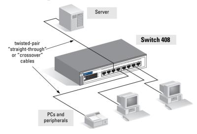
The Switch 408 is designed to be used primarily as a desktop switch to which end nodes, printers and other peripherals, and servers are directly connected, as shown in the above illustration.
