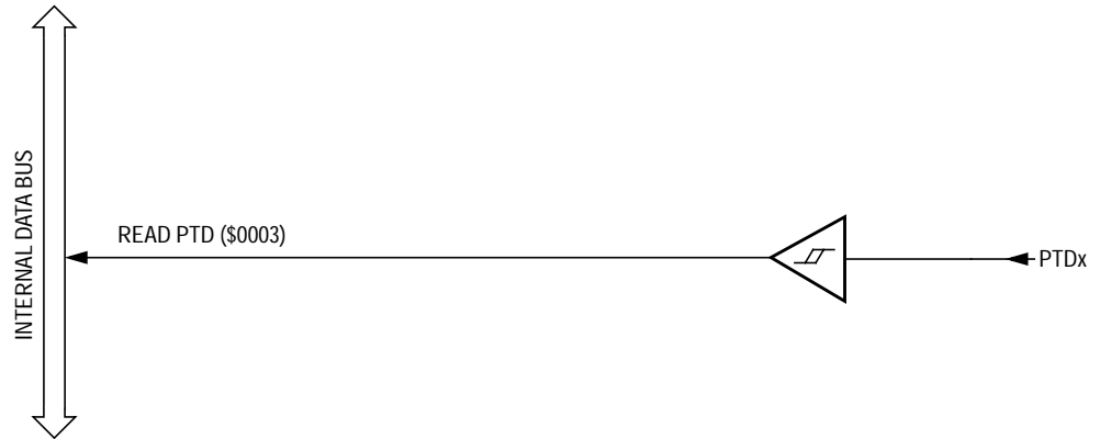
Figure 15-12. Port D Input Circuit
